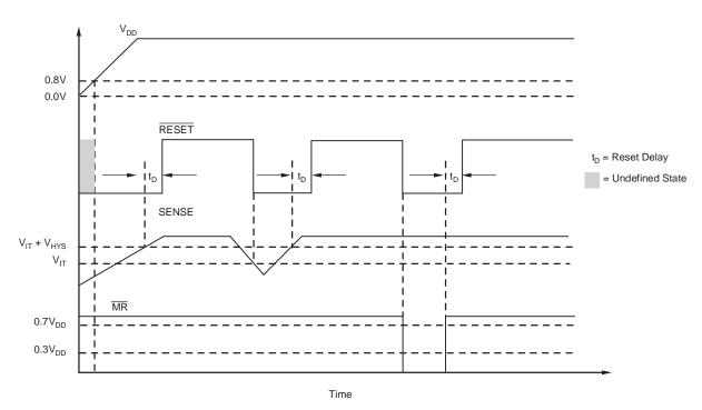
Figure 1. MR and SENSE Reset Timing Diagram
