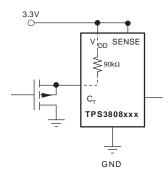
Figure 11. Using an External MOSFET to Minimize I<sub>DD</sub> When MR Signal Does Not Go to V<sub>DD</sub>
