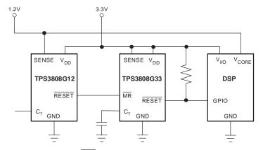
Figure 10. Using MR to Monitor Multiple System Voltages
