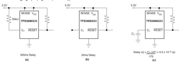
Figure 12. Configuration Used to Set the RESET Delay Time
